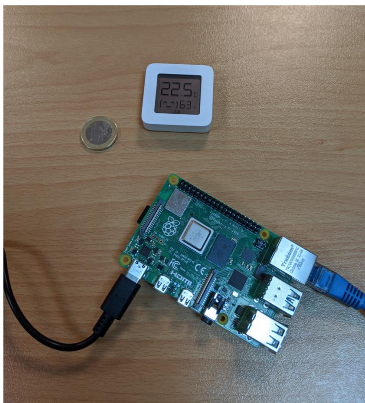
Figure 39. The temperature and humidity sensor wirelessly connected to Raspberry Pi.
